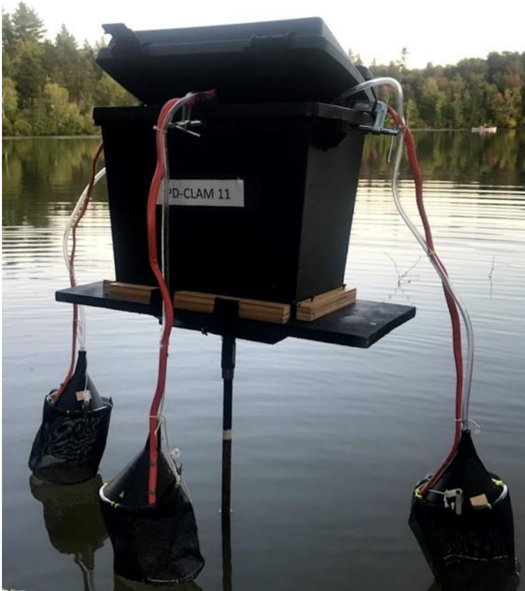
Figure 3. Compact Lake Aerosol Monitor (CLAM) set up on a temporary platform during a collection. Funnels and wind screens are positioned directly on the surface of the water. The three sets of filters, liquid traps, and pumps are inside the CLAM box.
